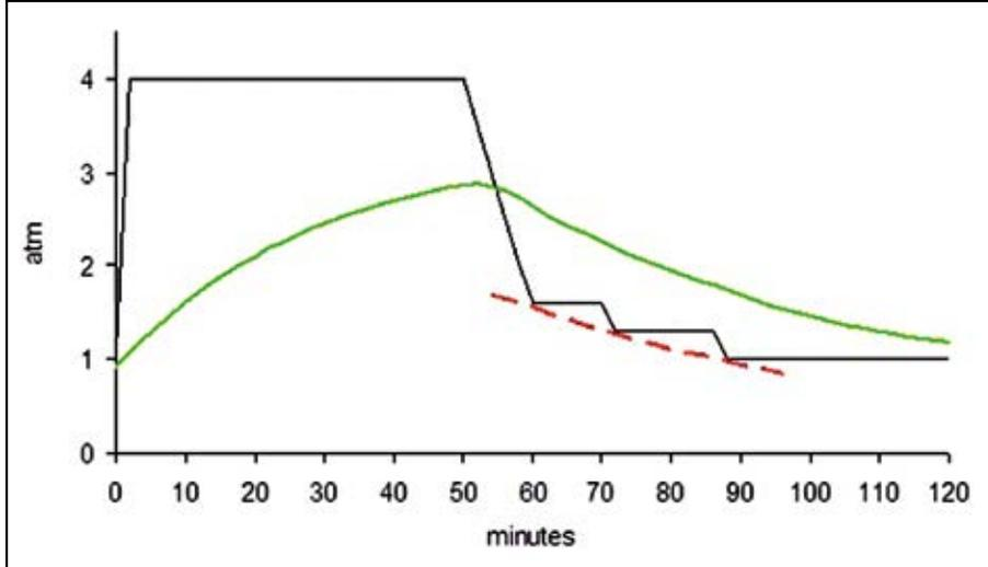
Figure 1. Exponential approach of tissue gas pressure ( $P_{tis}$ , green line) to arterial gas pressure (not shown) with changing ambient pressure ( $P_{amb}$ , black line) during a 100 fsw (30 msw) dive. The Haldane-style safe ascent depth is shown as a dashed line (see the gas content model section for explanation).
