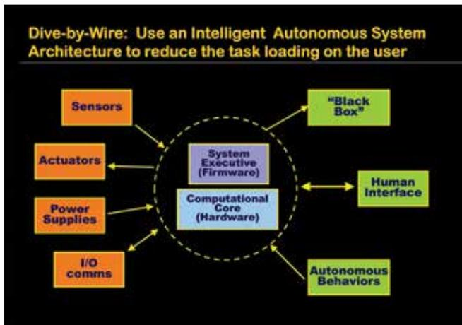
Figure 28. Block architectural chart for a “dive-by-wire” rebreather.
