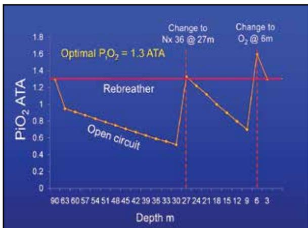
Figure 7. See text for explanation. An illustration of the contrast in  $PO_2$  during ascent when using a CCR versus open-circuit scuba with intermittent gas changes. Note how the  $PO_2$  constantly remains at 1.3 atm during the ascent on the rebreather but falls between gas switches during upward progress during ascent on open circuit.
