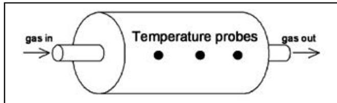
Figure 7. Illustration of temperature sensors in a CO<sub>2</sub> scrubber.
