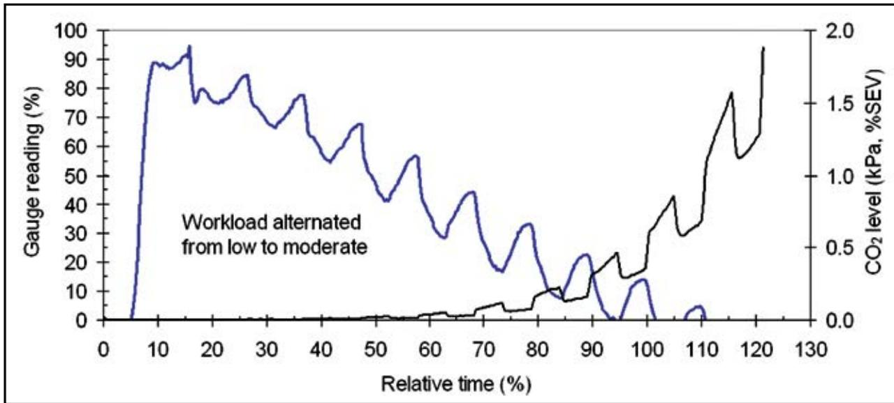
Figure 10. Variations in the scrubber gauge reading and CO<sub>2</sub> trace from a rebreather where the simulated diver workload varied.
