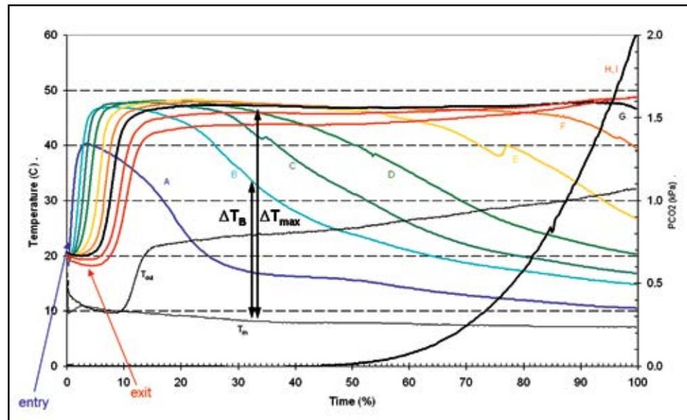
Figure 8. Temperature variations recorded from nine sensors placed in a CO<sub>2</sub> scrubber and the CO<sub>2</sub> in the inspiratory hose. Temperatures are shown on the left vertical axis and CO<sub>2</sub> level on the right vertical axis. Time is expressed as a percentage of the entire run; 100 percent does not mean the time to a physiologically acceptable CO<sub>2</sub> level.
