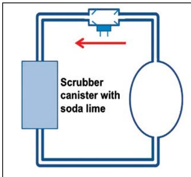
Figure 2. Simplified and stylized depiction of a basic rebreather circle circuit or “loop” with a CO<sub>2</sub> scrubber canister added.
