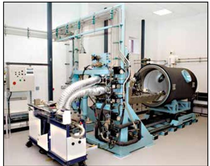
Figure 1. Unmanned test chamber and breathing simulator.
