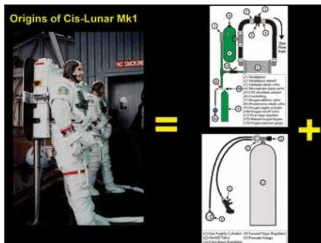
Figure 9. The space shuttle extravehicular mobility unit (aka “spacesuit”) and a simplified schematic of its internal life-support systems, which consist essentially of an oxygen rebreather and an open-circuit bailout.
