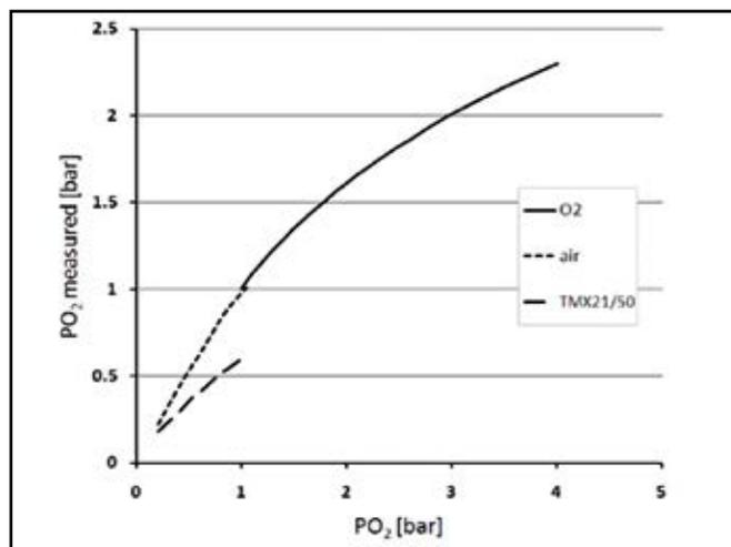
Figure 8. Characterization of the solid-state PO<sub>2</sub> sensors. Reprinted with permission of Diving and Hyperbaric Medicine (Sieber et al., 2011).
