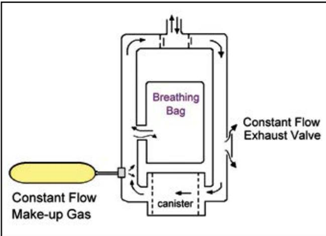
Figure 3. Schematic of the simplest mechanical semiclosed-circuit rebreather.
