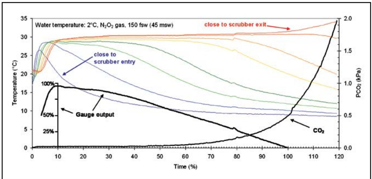
Figure 9. Temperature and CO<sub>2</sub> variations recorded from eight sensors placed in a CO<sub>2</sub> scrubber. The calculated gauge output is also shown.
