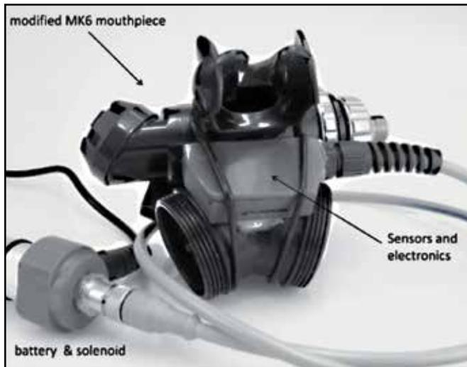
Figure 7. Modified rebreather mouthpiece with solid-state O<sub>2</sub> and CO<sub>2</sub> sensors. Reprinted with permission of Diving and Hyperbaric Medicine (Sieber et al., 2011).
