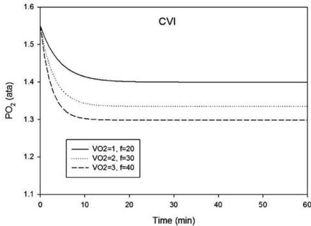
Figure 22. CVI rebreather PO<sub>2</sub> control for three levels of oxygen consumption and three respiratory frequencies (breaths per minute). John R. Clarke figure.
