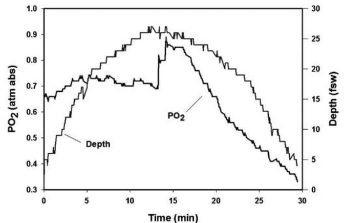
Figure 15. PO<sub>2</sub> and depth profile for an instrumented diver making a beach dive. John R. Clarke figure.
