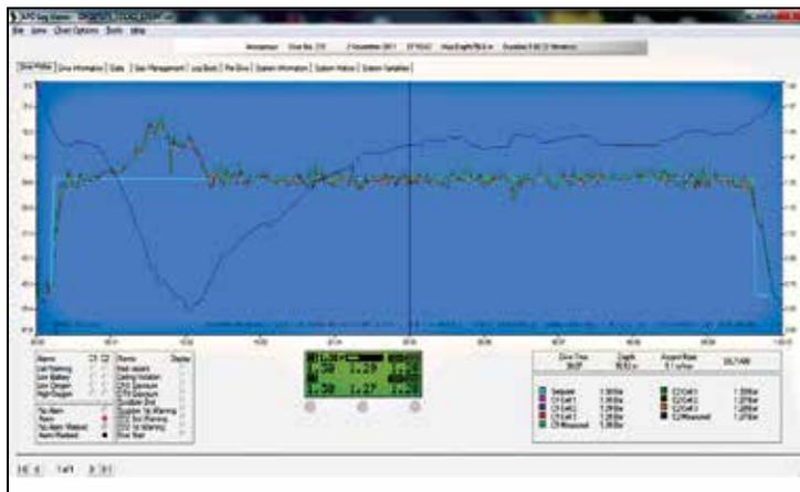
Figure 4. The LogViewer: PO<sub>2</sub> display, setpoint selection, solenoid activity, warnings.
