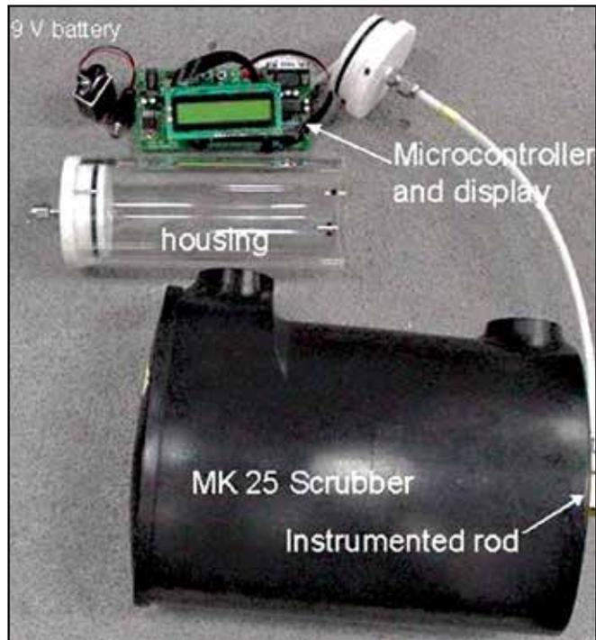
Figure 11. Photograph of the proof-of-concept unit developed for the U.S. Navy MK 25 100 percent O<sub>2</sub> rebreather. This unit was meant for verifications and demonstrations, not for field use.
