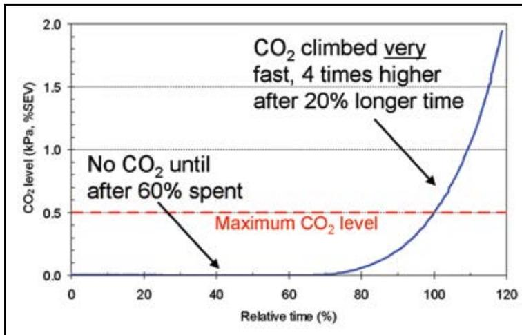
Figure 2. Common variations in the CO<sub>2</sub> levels measured in the inspiratory hose during a dive. The red, interrupted horizontal line indicates the maximum acceptable CO<sub>2</sub> level.
