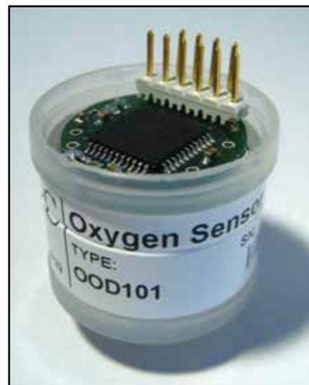
Figure 5. Prototype of our "smart" galvanic O<sub>2</sub> sensor.
