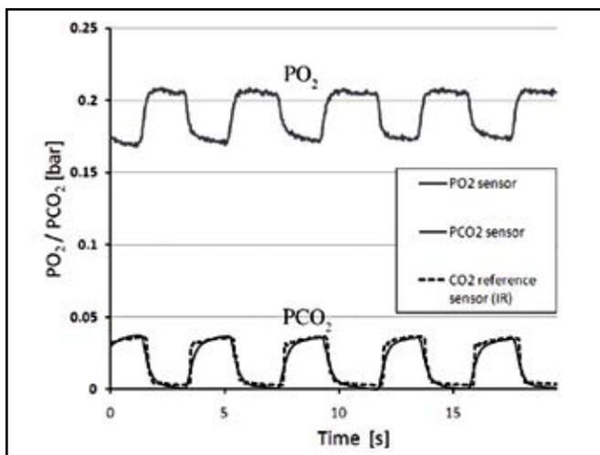
Figure 9: Sample breath-by-breath recording of  $PO_2$  and  $PCO_2$  from the transducer module in the rebreather mouthpiece. Reprinted with permission of Diving and Hyperbaric Medicine (Sieber et al., 2011).
