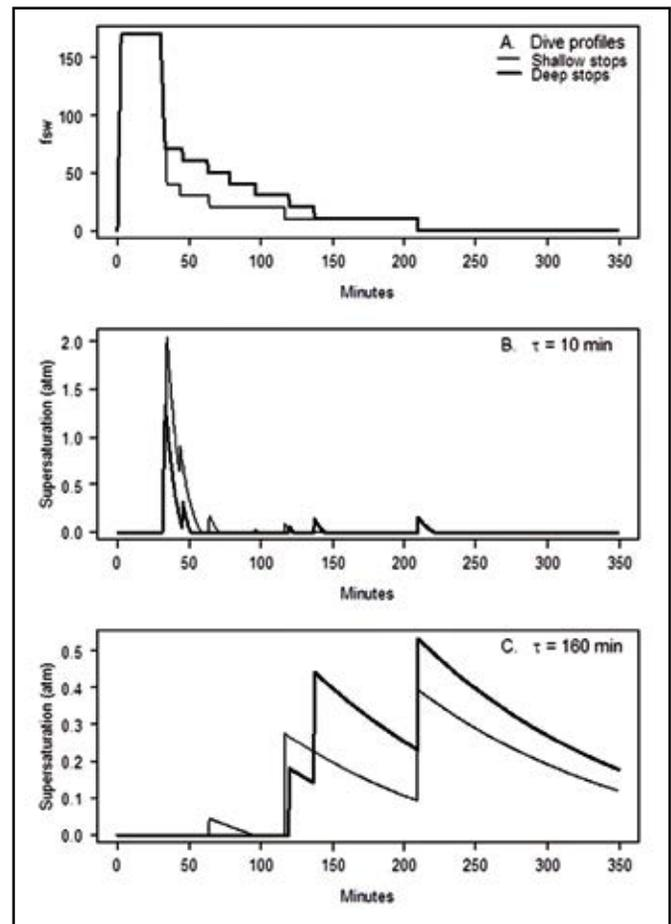
Figure 4. Supersaturation ( $\Sigma P_{tisj} - P_{amb} > 0$ ) in fast and slow compartments for the tested shallow-stops and deep-stops schedules. A. Overlay of the two 170 fsw (52 msw) / 30-minute air decompression dive profiles tested. B. Supersaturation in a modeled compartment with fast ( $\tau = 10$  minutes) mono-exponential inert gas exchange. C. Supersaturation in a modeled slow ( $\tau = 160$  minute) compartment. From Doolette et al. (2011).
