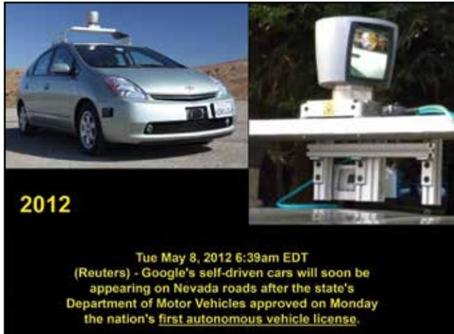
Figure 39. Google's self-driving car, used to automatically create "street views" for Google Maps.
