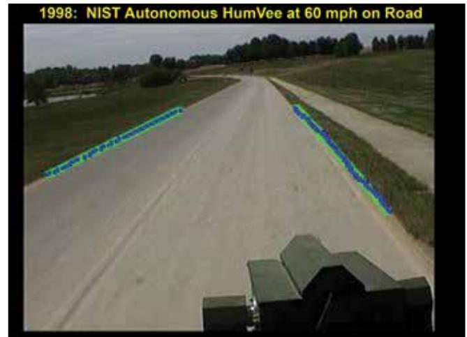
Figure 34. An illustration of machine vision serving as the “eyes” for an intelligent system (in this case, an unmanned ground vehicle).
