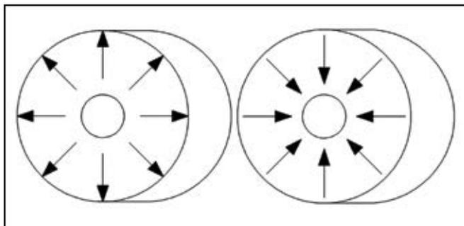
Figure 5. Illustration of two types of radial scrubbers.
