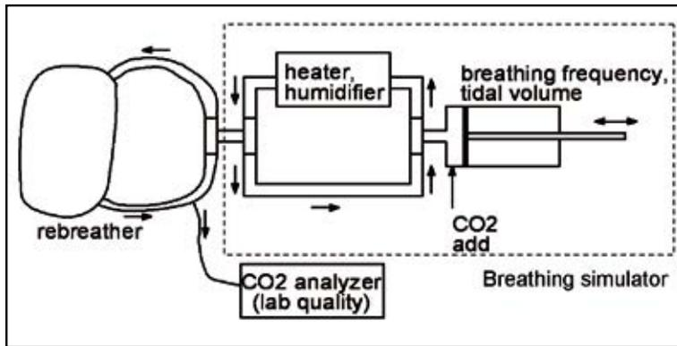
Figure 1. Schematic of the test set-up for determining the endurance of a CO<sub>2</sub> scrubber. The rebreather to be tested is on the left. The interrupted line encloses the parts of the breathing simulator. Arrows indicate the piston movement and gas movement, respectively.
