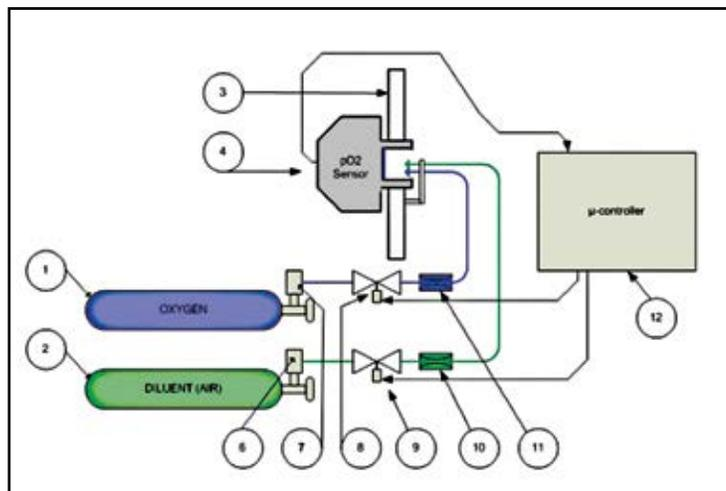
Figure 3. Schematic of our true PO<sub>2</sub> sensor signal validation system (1: O<sub>2</sub> tank; 2: diluent tank; 3: sensor support; 4: PO<sub>2</sub> sensor; 6, 7: pressure regulators; 8, 9: solenoids; 10, 11: flow restriction orifices; 12: microcontroller). Reprinted with permission of Diving and Hyperbaric Medicine (Sieber et al., 2008).
