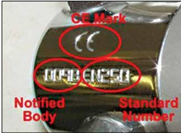
Figure 6. First-stage diving regulator showing CE marking.
