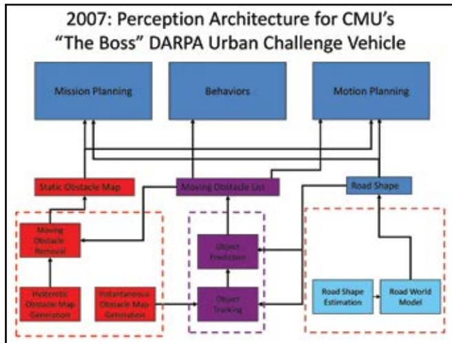
Figure 38. Perception architecture for an unmanned ground vehicle.
