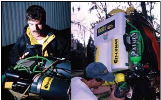
Figure 21. Final kitting up with the dual backmounted rebreather, January 1999. The small green tank is offboard oxygen; the small yellow tank is drysuit inflation argon supply. A second oxygen tank was placed inside the shell between the two CO<sub>2</sub> canisters.
