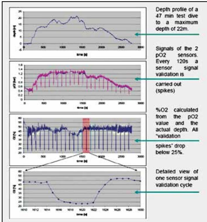
Figure 4. Data from a 100-minute test dive (6,000 seconds) in the Mediterranean Sea to a maximum depth of 22 m (72 ft). (A: depth profile; B: PO<sub>2</sub> sensor signals of two sensors; C: calculated fO<sub>2</sub>; D: one validation cycle) Reprinted with permission of Diving and Hyperbaric Medicine (Sieber et al., 2008).
