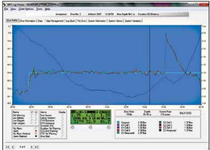
Figure 5. Computer record from a fatality in which there was a spike in PO<sub>2</sub>.
