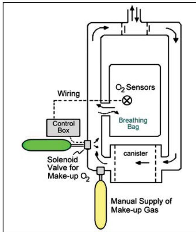
Figure 2. Schematic of an electronically-controlled mixed-gas rebreather.
